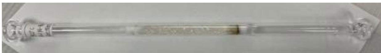
*Figure 4. Catalyst bed in reactor*
